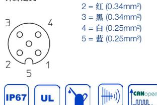
5 针 M12x1 凹直接头, A 型, IP67
